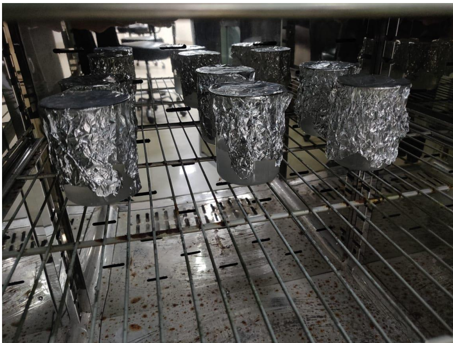
Figure 3.6: Digestion with 30% H 2 O 2 in drying oven
