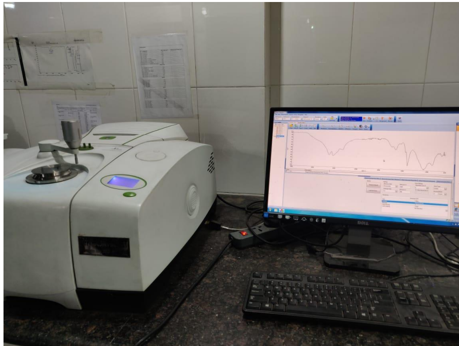
Figure 3.8: Chemical analysis of MPs using FT-IR spectroscopy
