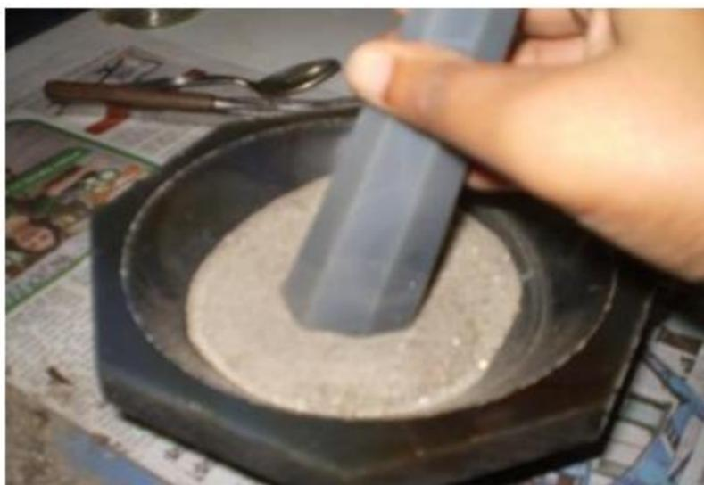
**Figure 3.5 Grinding of the samples**
