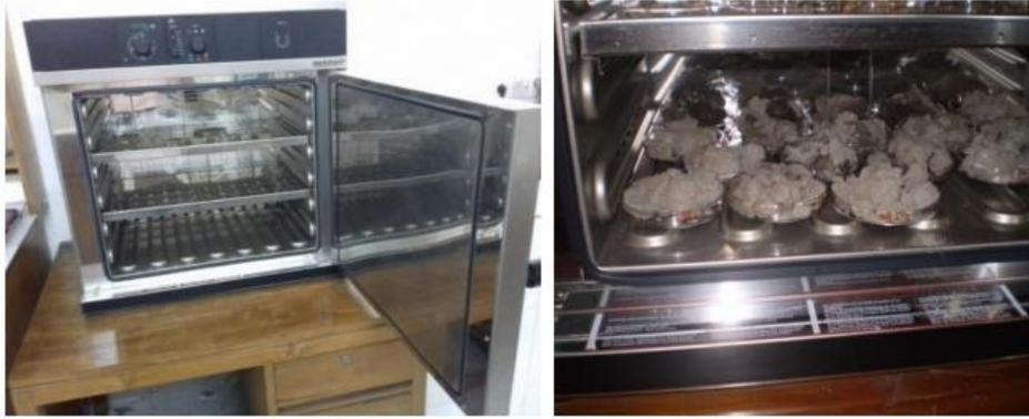
**Figure 3.3 Sample drying in micro-oven**
